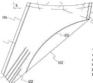
The cone is a collapsed funnel which by way of apatented arrangement of score marks when pressed on at a specific point at the bottom of the cone in its collapsed state pos open into arigid cone which locks in place, maintaing its rigidity during use.
